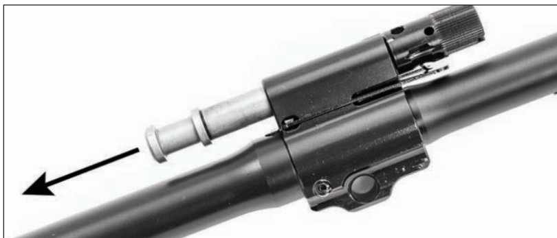
Fig. 26 – Removing Gas Piston
