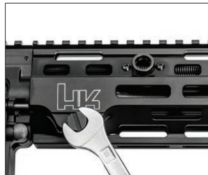
Fig. 23 – Loosening the screw on MR556 A4 handguard with 11mm wrench
