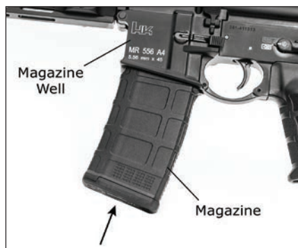
Fig. 16 – Insert loaded magazine into the magazine well
