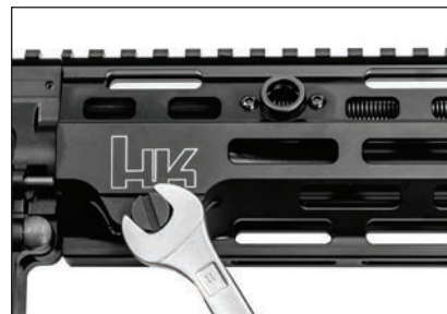
Fig. 51 – Tightening the locking screws on the MR556 A4
