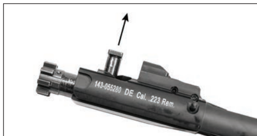
Fig. 21 – Remove the Cam Pin
