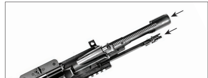
Fig. 38 – Installing the bolt carrier assembly into the upper receiver
