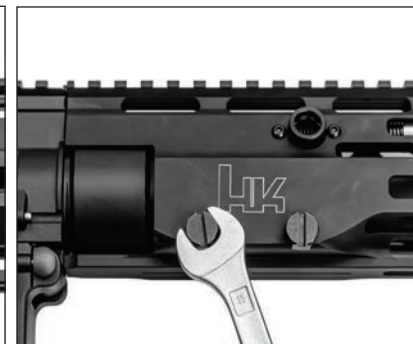
Fig. 24 – Loosening the screws on MR762 A4 handguard with 11mm wrench
