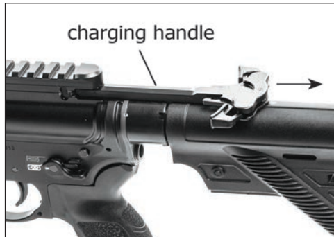
Fig. 8 – Pull the charging handle rearward
