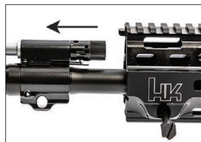
Fig. 49 – Slide the handguard over the barrel to install
