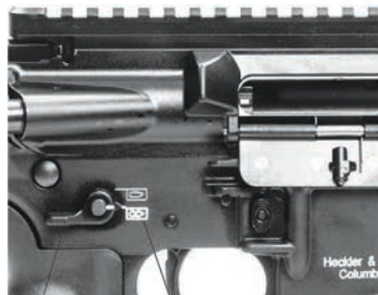
Safety/Selector Lever SAFE position
