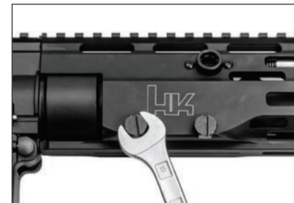
Fig. 52 – Tightening the locking screws on the MR762 A4
