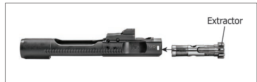
Fig. 33 – Bolt Carrier reassembly
