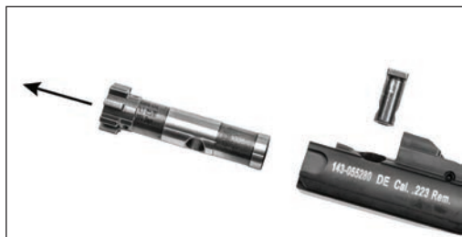
Fig. 22 – Slide the Bolt Head out
